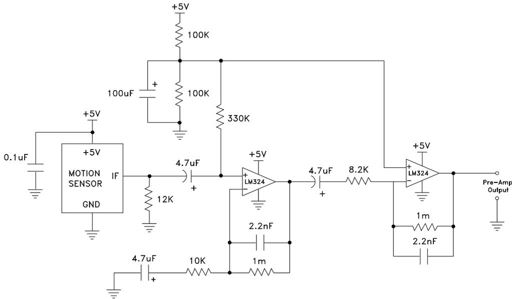
Amplifier Circuit (Pulse operation, PRF=2 KHz, Duty Cycle=4%)
